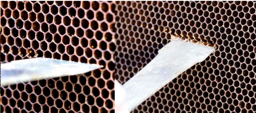
2. Starting the notch by cutting
